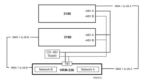
Figure 3. Recommended Network Setup for 3190 Type Shelves
